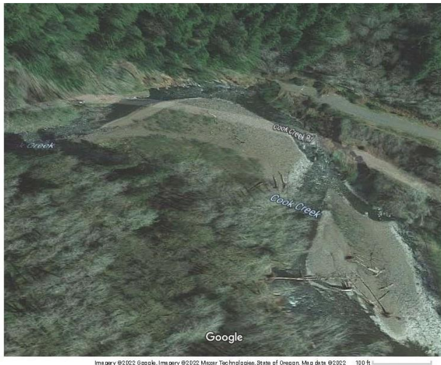
Google Earth, Cook Creek Road wash-out looking north. The outside bend of the stream (near the top of the image) is against the hillside and directly underneath the former road location.
